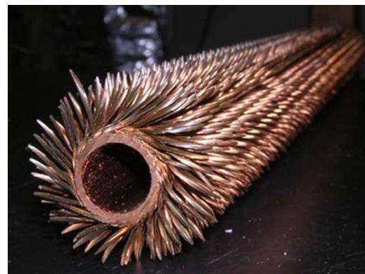
Fig. 3 Photograph of the spined copper pipe used as the inner tube in the double-pipe heat exchanger
